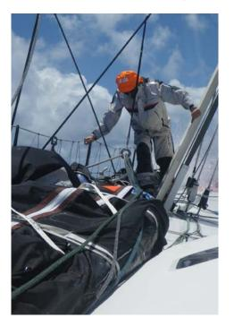
In order for a boat to sail as quickly as possible, it has to sail flat, not too far over on its side. To counteract the forces of the wind that heel the boat over, naval architects use a number of tricks including swinging keels and ballast tanks. For their part, the sailors have the tough job of trimming the moveable ballast onboard. Basically this means moving anything that's not fixed down from one side to the other as the boat changes tack, and that includes cabin and deck gear!
